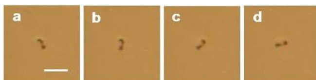
Fig. 3 Co-rotation of defect pair slightly below the threshold field after the ER to split transition occurred. Approximately 33 ms separate successive images. Scale bar corresponds to 15 \mu\text{m} .
