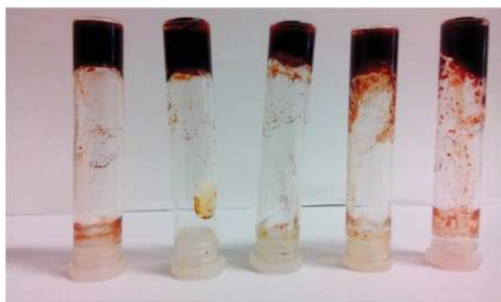
Fig. 6 Cu(II):L1 (8 mM/8 mM) Gels in presence of 8 mM NaCl after dissolving L1 in HNO 3 , H 2 SO 4 , HBr, HClO 4 and p -toluenesulfonic acid (left to right).
