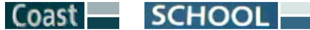
Figure 4. Two detected and automatically rectified text areas with estimated foreground and background color on their right side.
