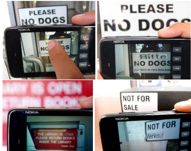
Figure 1. TranslatAR in operation: the user detects a word he/she wishes to translate and taps on it (top left). The system automatically detects the extent of the word, extracts the letters via OCR, and translates the text. The translation is then presented as live AR overlay (top right). Bottom row: TranslatAR used in two other situations.
