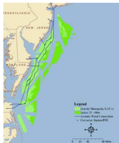
FIGURE 1. Potential wind power plant development areas. Green Areas: offshore wind power plants up to 60 m water depth and excluding use conflicts [17] [24]. Black Lines: HVDC backbone proposed by Atlantic Wind Connection, LLC [7], with Point of Interconnections (POIs) shown as dots.
