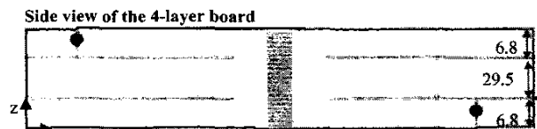
(b). Geometry of FDTD modeling for the 4-layer board.
