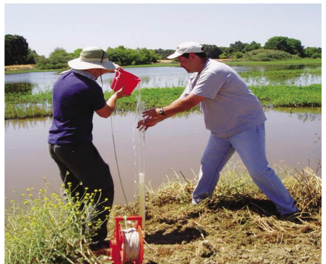
UC Davis graduate student John Maynard (left) and UC Cooperative Extension specialist Toby O'Geen examine the effects of wetland treatment for water-quality improvement of irrigation tailwaters in western Stanislaus County. As shown by the transparency tube, suspended solids are effectively removed by treatment in flow-through wetlands. The transparency tube provided accurate measurements of water transparency, and is a low-cost tool that is easy to use in the field.
