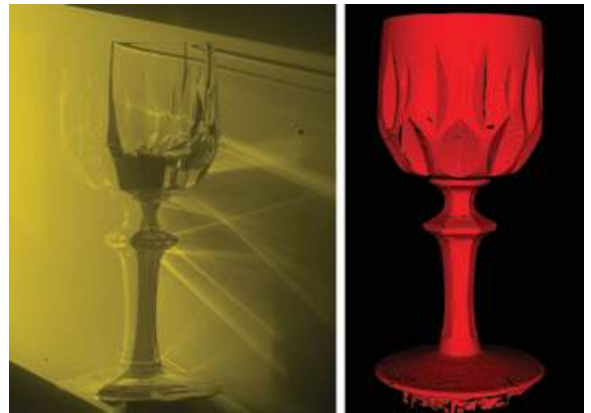
Figure 2: Left panel: surface scanning of glass objects [HFI*08] by detecting laser sheet cut-off instead of the laser reflection off the object's surface. Right panel: resulting range scan.
