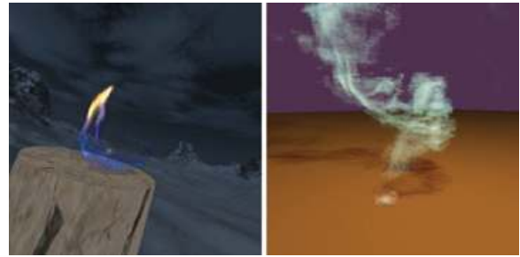
Figure 16: Results of tomographic reconstruction on fire [IM04] (left panel) and smoke data sets [IM05, IM06] (right panel). The multi-view setup used to capture the input data consists of 8 cameras, Reconstruction resolution is 128^3 (left panel) and an octree-representation with effective resolution of 256^3 (right panel).
