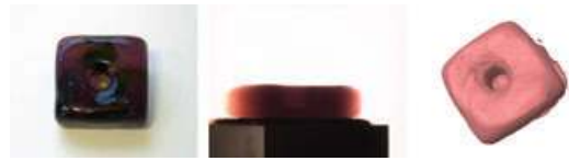
Figure 13: A photograph of a refractive object with absorptive properties (left), a tomographic projection obtained by matching the refractive index of a surrounding medium to the one of the object (middle) and the object's surface generated by iso-surface extraction on a volumetric representation of the absorption density of the object (right). The absorption density is reconstructed by tomographic means [TBH06].
