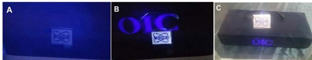
Figure 16. (A) Scattering of blue light from the whole transparent screen, (B), projecting OIC logo on transparent display and (C) projecting OIC in white light ambient.
