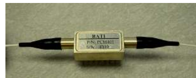
Figure 13. Schematics of a polarization controller design and an Acrobat™ polarization controller.
