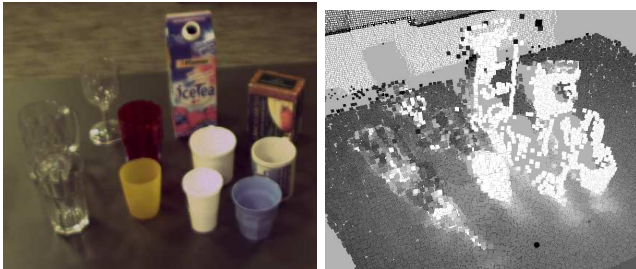
(a) Camera image of the objects illuminated by laboratory light with a high proportion of green. (b) ToF point cloud of the objects.
