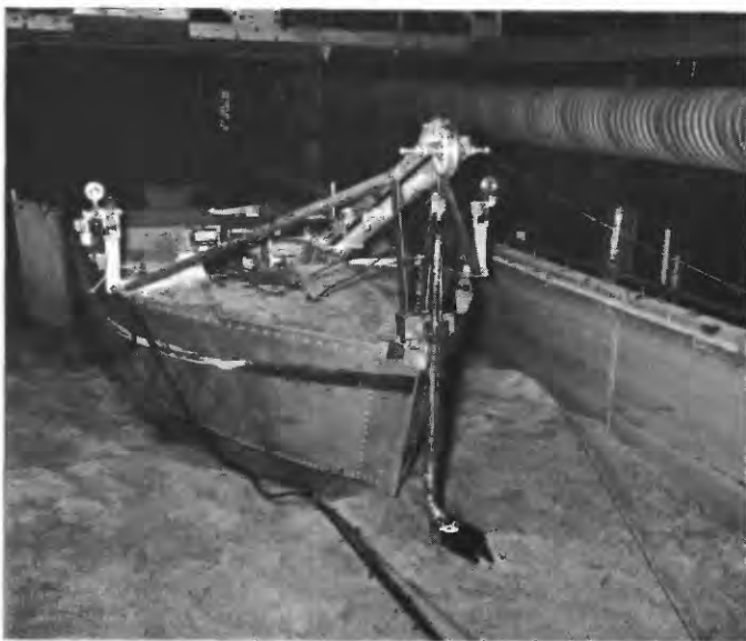
FIGURE 12.—Dual ultrasonic depth sounder and distance-marking system.
