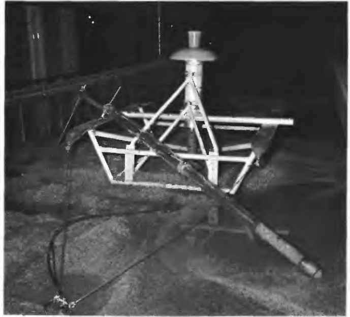
FIGURE 13.—Equipment for sampling and analyzing the bed material. The 1½-inch-diameter sampler is used to collect 3-foot cores, which are ejected in 2-inch-increments with the hand jack attached to the end of the sampler plunger. Samples are counted with the detector and sled in an inverted position.
