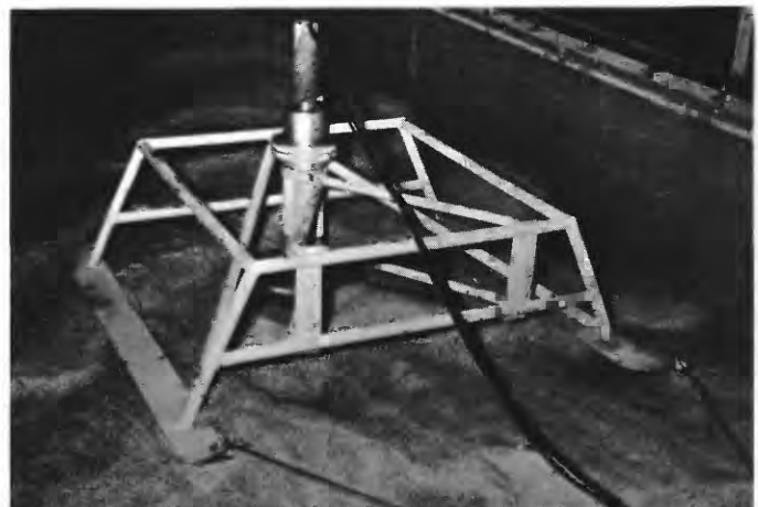
FIGURE 8.—Sled and scintillation detector. Note the parallelogram linkage, which allows the detector to move independently from the sled, and the wooden dish-shaped piece that supports the detector on the bed.
