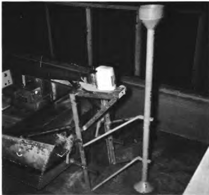
FIGURE 6.—The dosing apparatus. Note the tongs used for handling the cans of labeled sand and the adjustable mount with parallelogram linkage, which permits the funnel tube to be raised and lowered vertically.
