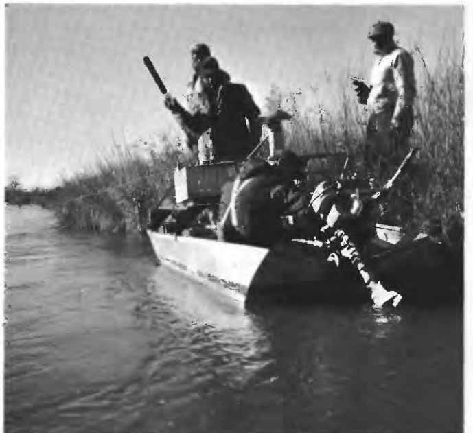
FIGURE 14.—Analysis of the vertical distribution of labeled particles in the field. Note the scaler and the inverted detector sled on top of the canopy over the instruments.
