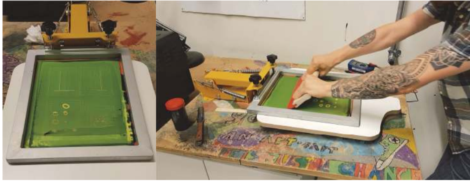
FIGURE 6: Left: screen-printing frame with exposed design. Right: screen-printing of EC displays.
