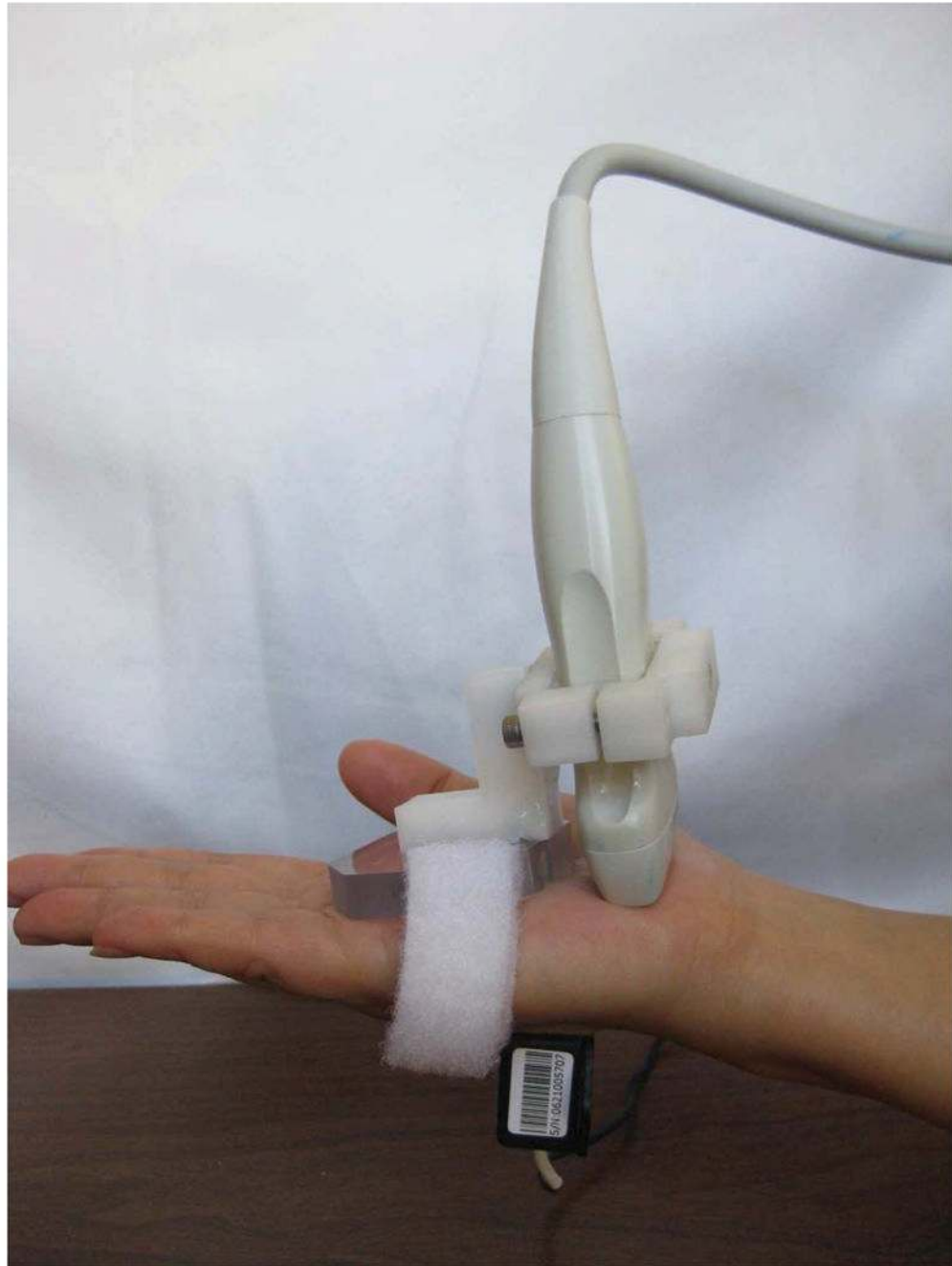
Figure 1. Ultrasound examination setup. The transducer was placed at the proximal carpal tunnel. A custom-made transducer-fixing device was fastened at the subjects' palm to keep the transducer stable during finger or wrist motion. A goniometer was fixed on the back of hand to measure the wrist angle during wrist movement.
