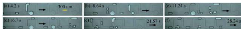
Fig. 3 Experimental results showing generation of the guiding bubble. The arrow indicates the flow direction. (a)–(f) The generation of the bubble at different times. The time when the long bubble just enters the first junction of the MTN is defined as 0 s. The trapping unit no. of (a)–(d) are 1, 2, and 3. The trapping unit nos of (e) and (f) are 3, 4, and 5.
