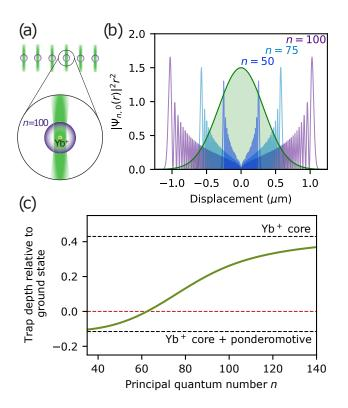
FIG. 1. (a) Cartoon of the experiment, showing a six-tweezer array, the Rydberg electron wavefunction, and the Yb<sup>+</sup> ion core. (b) Radial probability distributions of Rydberg wavefunctions relative to the optical tweezers (green). (c) Calculated trap depth for  ${}^{3}S_{1}$  states, normalized to the trap depth for the  ${}^{1}S_{0}$  ground state for the same power and beam waist (here, 0.65  $\mu$ m).
