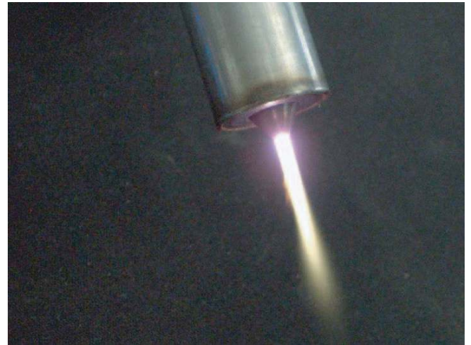
FIG. 2: Picture of a nitrogen plasma torch in operation. The plasma plume is 4 cm long and the diameter of the torch itself is 2 cm.
