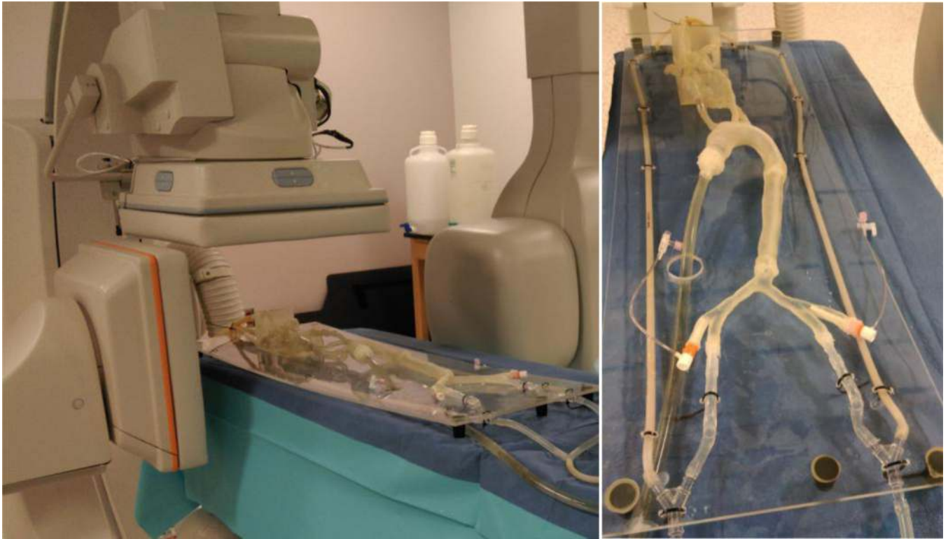
Figure 4. Several printed phantoms put together to better simulate the traversal of the catheter from the entry point in the femoral artery to the treatment site.
