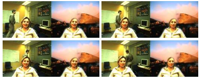
Figure 11. Background substitution on the “IU” test sequence from [8]. Original and corresponding segmented frames with background substitution. People moving behind the foreground person are correctly classified as background.
