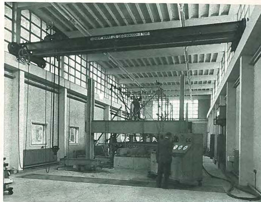
Fig. 3. General view of the interior of the structures' laboratory showing the test frame with bridge decks in position for testing. The hydraulic console is shown in the foreground.
