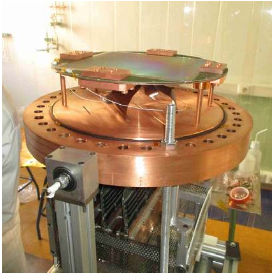
Fig. 4 View of one of the vessel's caps, where several components described in detail in the text are shown: a readout plane, its copper shielding pieces, its four flat cables and part of the electronics: the interface cards and the FEC cards
