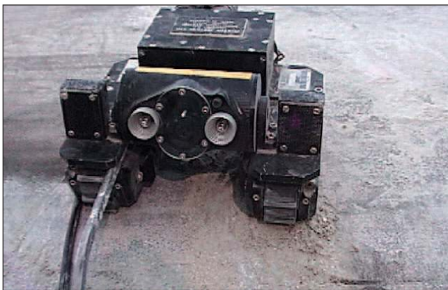
Figure 8. Metal rod jammed between the tracks and housing on an micro-Tracs robot.
