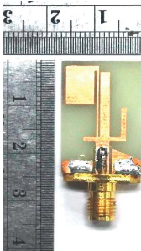
FIGURE 10: Prototype of the WLAN/WiMAX triband antenna.
