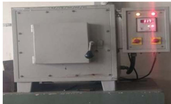
FIGURE 1: Heat treatment by muffle furnace KSM-0012.
