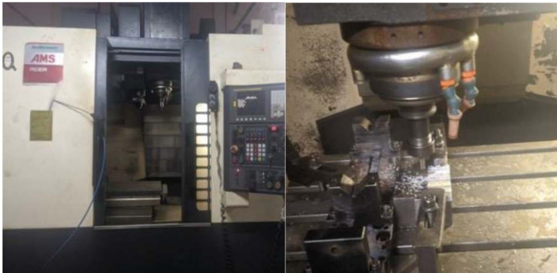
FIGURE 2: Experimental setup in CNC milling machine.
