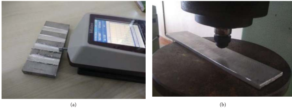
FIGURE 3: (a) Measurements of Ra on machined slots with Mitutoyo surface roughness tester. (b) Hardness measurement in the Rockwell hardness setup.
