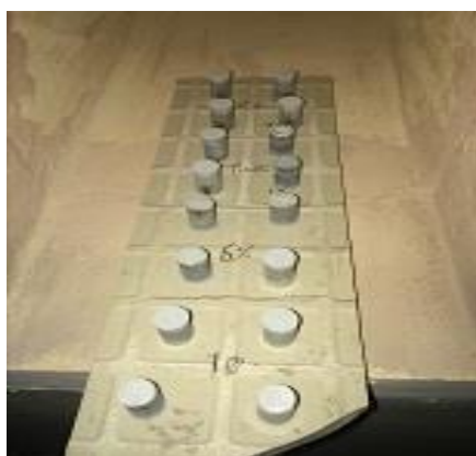
Fig. 3. Sintered specimens with SiC wt.% (3, 7 and 10).
