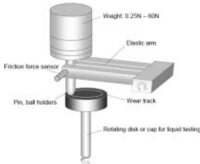
Figure 1 The pin-on-disk tribosystem (schematic arrangement)
