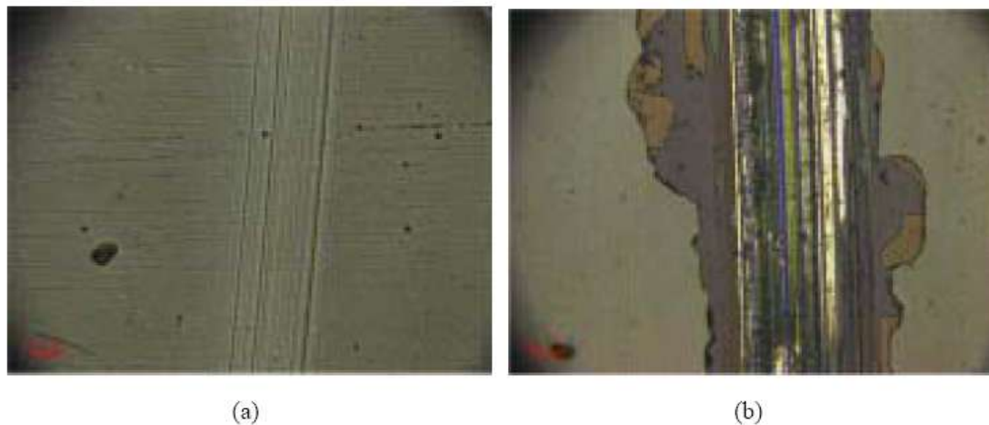
Figure 6 Micrographs of the wear tracks for the films with (a) the highest C content ( \text{TiC}_{7.3}\text{O}_{0.56}\text{N}_{1.14} ) and (b) the lowest C content ( \text{TiC}_{1.8}\text{O}_{0.27}\text{N}_{0.36} ) (see online version for colours)
