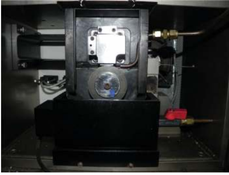
FIGURE 2: Close-up view of specimen loading in multitribotester.
