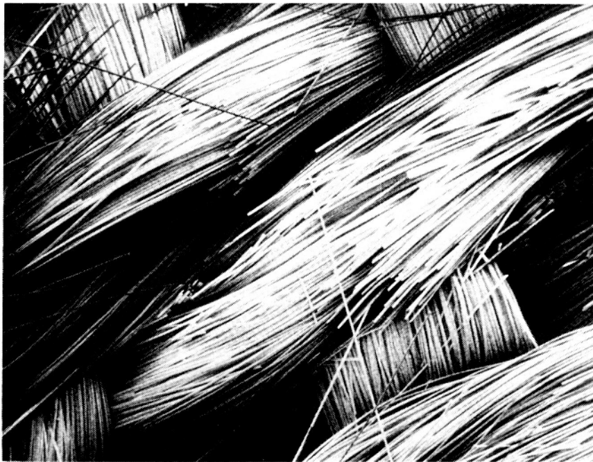
FIGURE 8. - FABRIC FRACTURE AFTER SLIDING AGAINST INCONEL X750. NO LUBRICANT COATINGS APPLIED. (TOP PHOTO 10X, LOWER PHOTO 50X.)
