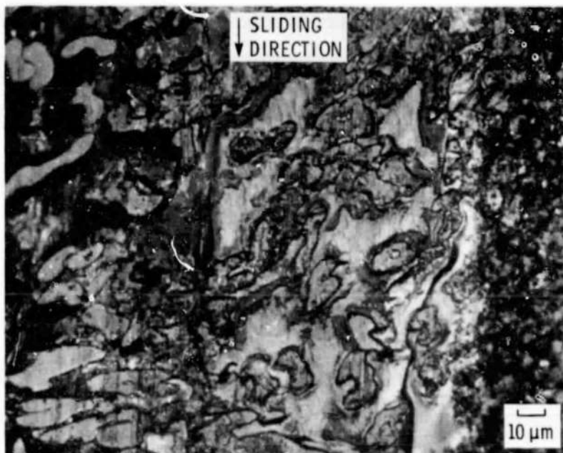
Figure 9. - Photomicrograph of wear surface of 60/40 PMDA/BTDA polyimide reinforced with type B fibers, after 3 km of sliding at 300 °C.
