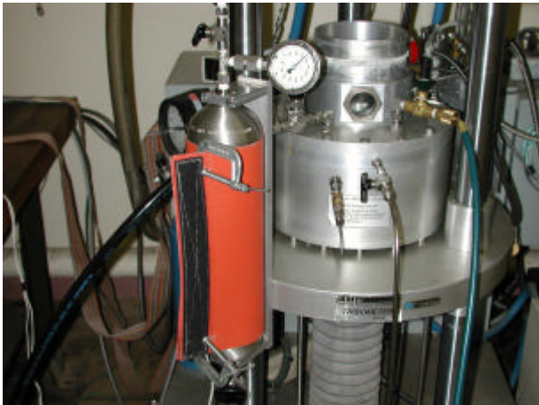
Figure 2.12 - Heating of the Pressure Vessel
