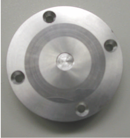
Figure 3.19 - Microscope Image of Al390-T6 Disk: Sample C (t = 22 min)
