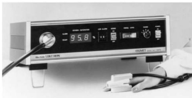
Fig. 6 OXIMET Met 1471. The light emitted by a light emission diode travels to the finger probe and the transmitted light is analyzed by a silicon photodiode mounted in the chassis. The incident and transmitted light travels to and from the chassis through the fiber-optics, respectively
