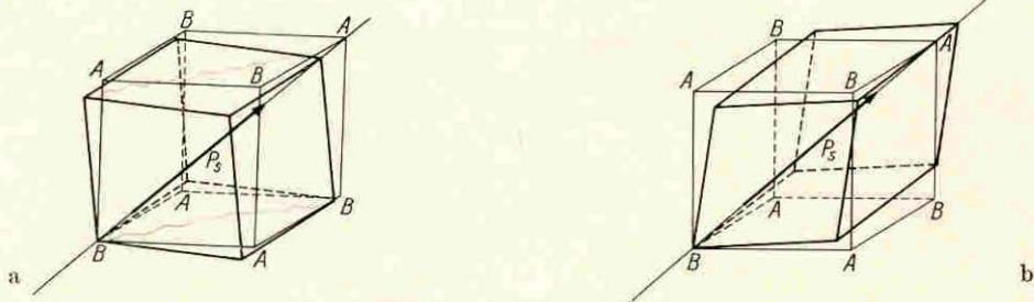
Fig. 2. Pseudo-cubic trigonal cell. a) Compressed along \mathbf{P}_s ; b) elongated along \mathbf{P}_s
