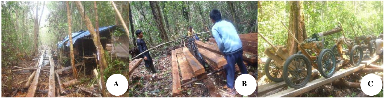
Figure 2. Low-impacted logging (A) and wood transportation using 'sepeda' (B) and 'gerobak' (C) on Ketapang, West Kalimantan peatland forest
