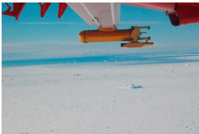
Figure 3. An airborne cloud probe mounted on a British Antarctic Survey aircraft observing clouds over the Antarctic Peninsula.
