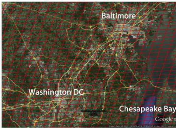
Fig. 2. TEMPO footprints overlaid on the Baltimore-Washington metropolitan area. The footprint size here is approximately 2.5 km N/S × 5 km E/W. Map created using Google Earth/Landsat Imagery.
