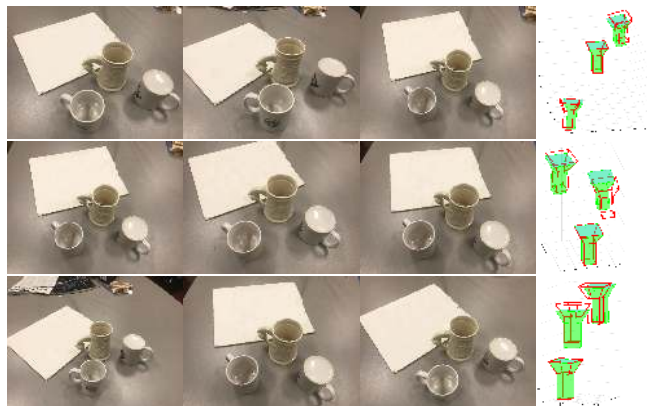
Figure 11. Trifocal relative pose results for a dataset comprising three mugs, which is challenging for traditional SfM. For each row, image triplet samples are shown, with results on the right. Ground truth poses are in solid green and estimated poses are in red.
