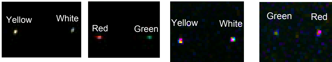
(a) Liquid Crystal Filter Camera (b) EMCCD/mosaic filter Camera Figure 13. Images taken with the TCNV cameras in a simulation of navigation lights at a distance.
