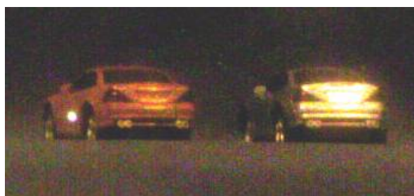
Fig. 2. Image taken with OKSI's TCNV camera demonstrating the ability to produce color imagery while utilizing both visible and NIR signal for brightness. The bright spot on the red car is from an NIR laser aiming device.
