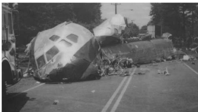
Fig. 1 Remnants of the aircraft N954VJ involved in USAir Flight 1016 [141]. The plane crash was attributed to the lack of warnings about wind shear from the air flight controller on duty who, due to mistrust in the wind shear alert system, reported only one out of three alerts generated by the system
