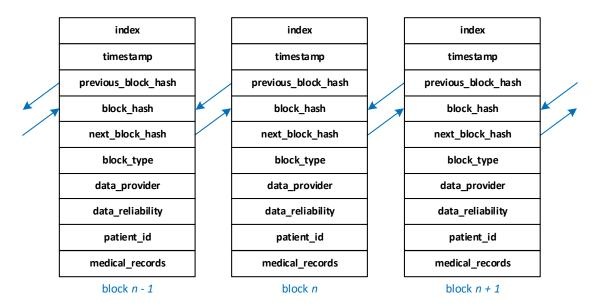
Figure 4. The proposed structure of the blockchain.
