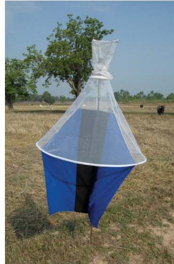
FIGURE 4: Vavoua trap. A trap designed for tsetse flies, especially efficient for Chrysops and Stomoxys .
