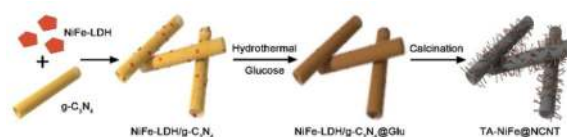
Scheme 1 Schematic illustration of the preparation process of TA-NiFe@NCNT.
