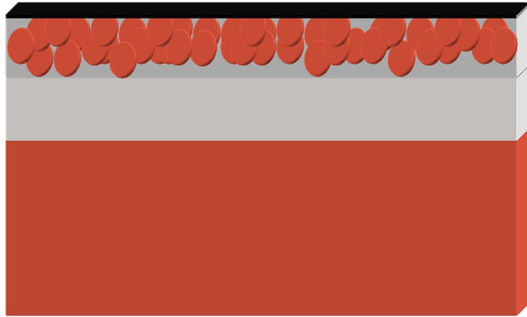
Figure 1(a): Schematic draw of the perfect absorber structure
