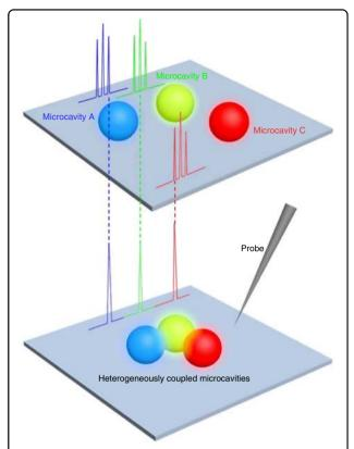
Fig. 1 Mode selection concept in the heterogeneously coupled resonant cavities. Sketch of the multimode lasing from isolated microspheres (top), and RGB single-mode lasing from heterogeneously coupled microcavities (bottom), where each microsphere functions as not only the laser source but also the mode modulator for the other resonators.
