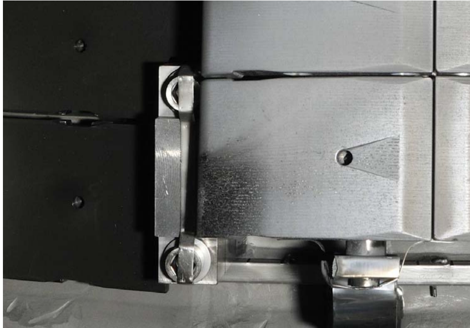
Fig.4 Local damage to W coatings at the bottom of the inner wall limiters which is due to the impact of runaway electrons
