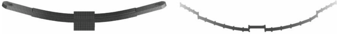
Fig. 7 1st bending mode of the finite element model ( left ) and the experimental modal analysis ( right ) at 167 Hz
