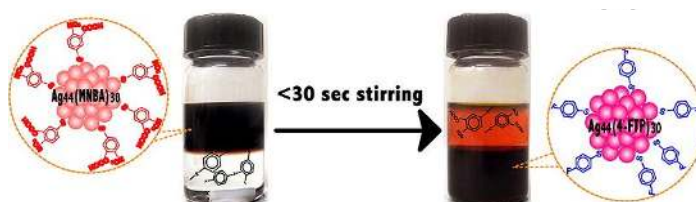
Figure 4. Phase transfer of aqueous [\text{Ag}_{44}(\text{MNBA})_{30}]^{4+} clusters into dichloromethane (DCM) using HSPHF as a ligand and tetraphenylphosphonium bromide (TPPB) as a counter-ion. 43 Reprinted from ref. [43] with written permission.
