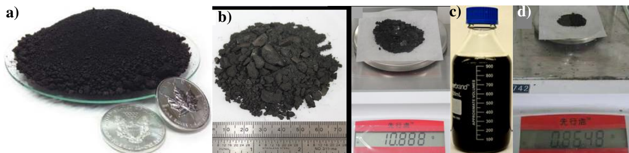
Figure 2. Scaled-up final single-sized product of a) [\text{Ag}_{44}(\text{p-MBA})_{30}]^{4-} , 140 g 28 ; b) [\text{Ag}_{44}(\text{SPhF})_{30}]^{4-} , 10.89 g 29 ; c) [\text{Ag}_{44}(\text{MNBA})_{30}]^{4-} clusters, 172 mg in 1 L of 1 M aqueous NaOH 48 ; and d) \text{Au}_{25}\text{Ag}_2(\text{PET})_{18} alloy cluster, 0.86 g 49 . Adapted from refs.[ 28-29, 48-49 ] with written permission.
