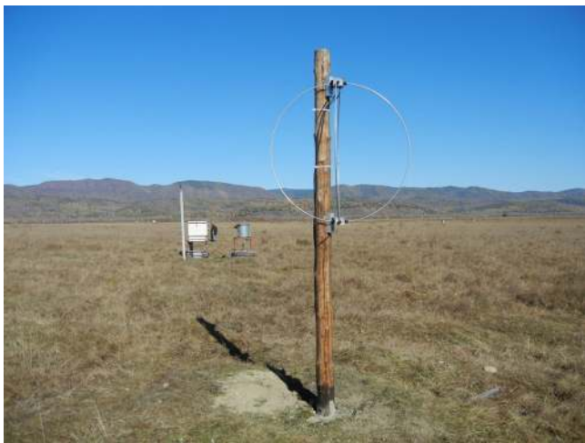
Fig. 2. A Tunka-Rex antenna in front of a Tunka-133 cluster center box and its central PMT.
