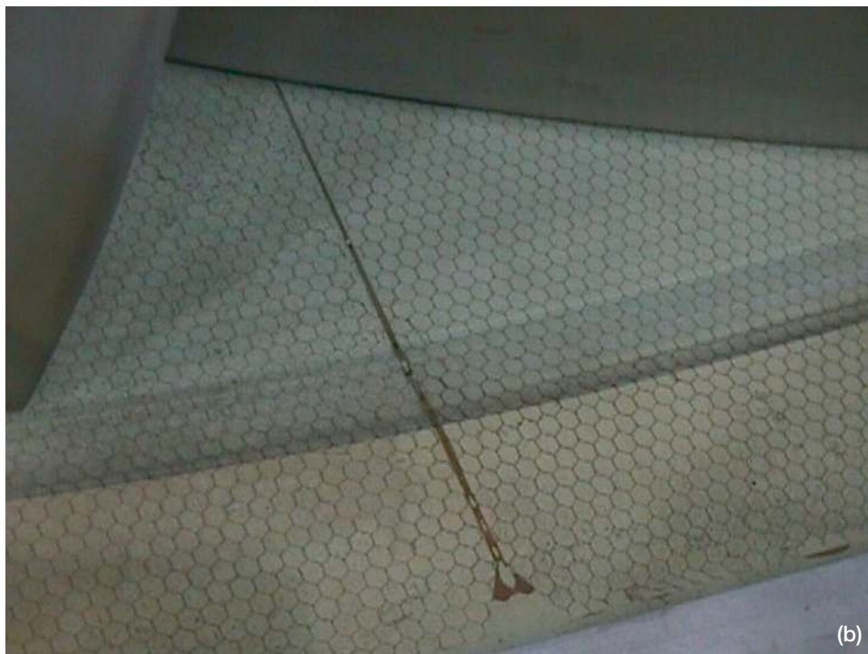
Figure 29.—PW4090 fan and rub strip. (a) Fan and shroud. (b) Fan/rub strip interface. (c) Rub strip. Courtesy Sherry Soditus, United Airlines Maintenance, San Francisco, CA.
