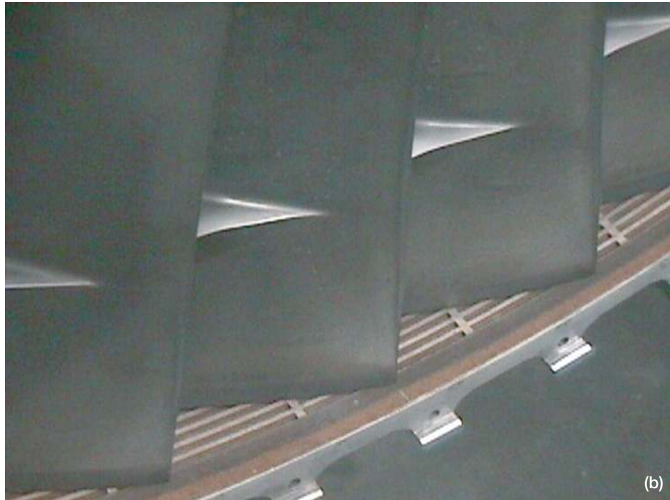
Figure 30.—PW2000/4000 fan rub strip. (a) Fan and shroud. (b) Fan/rub strip interface. (c) Rub strip. Courtesy Sherry Soditus, United Airlines Maintenance, San Francisco, CA.
