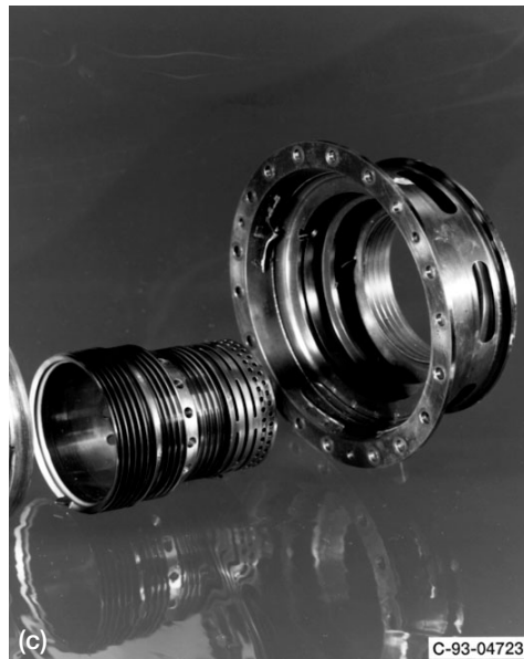
Figure 9.—Labyrinth compressor discharge pressure (CDP) seal. (a) Engine airflow and seal location. (b) Labyrinth seal package and airflow. (c) Simulated exploded view of labyrinth compressor discharge seal system. (Hendricks et al., 1994.)
