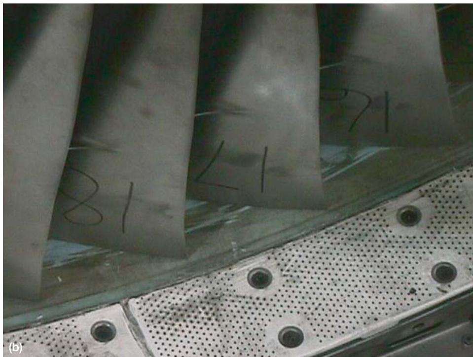
Figure 31.—CFM56 fan and rub strip. (a) Fan overview. (b) Fan/shroud interface. (c) Fan rub strip. (d) Closeup of fan rub strip. Courtesy Sherry Soditus, United Airlines Maintenance, San Francisco, CA.
