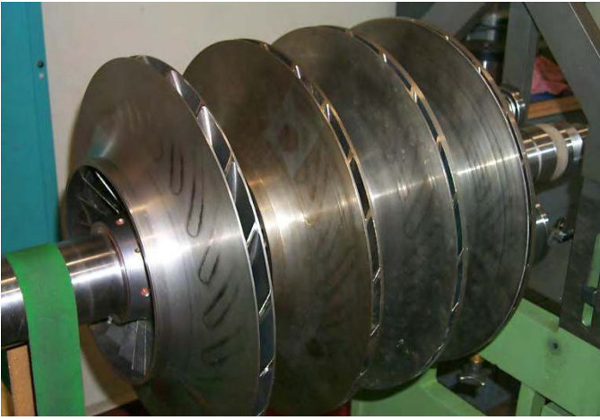
Figure 7. A rerated process compressor redesign; modeling demands are highly constrained: Impeller diameter and passage widths are specified a priori .
