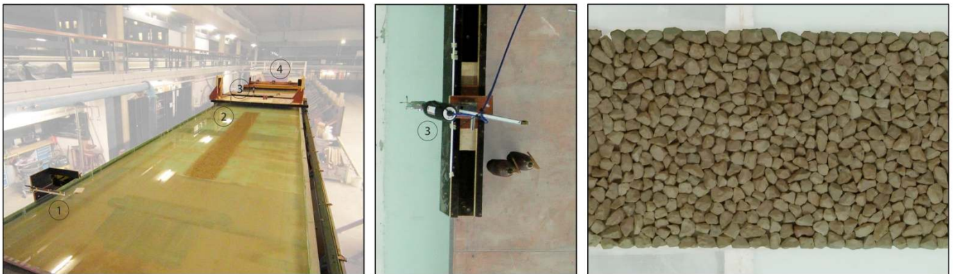
Figure 7; Schematic overview of layout experiment; 1) Electronic measurement of water level; 2) manual measurement water level; 3) ADV, 4) adaptable weir.
