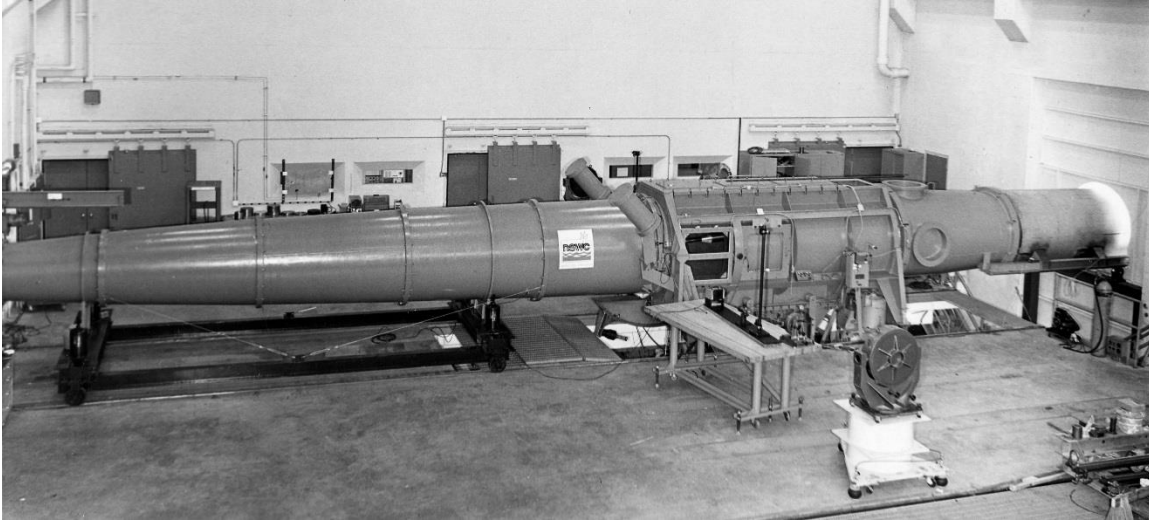
Figure 2.13: AEDC Tunnel #9. The tunnel is optically accessible using two sets of rectangular windows on the side of the test section. In this photograph, the downstream windows have been replaced with metal plates. In this research, the instrument presented here was installed on the upstream windows, while the downstream windows were used with the facility's schlieren system.
